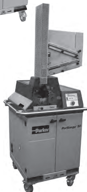
Parflange® 50 PRO for mass production of O-Lok® assemblies
