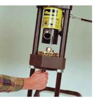
4. Move the hose fitting into the die set from below.
