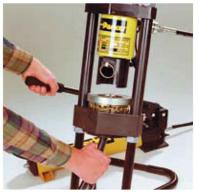
6. Position cylinder and replace pin. Pump until die ring contacts base plate.
