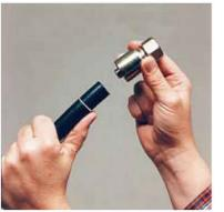
1. Mark the length of the shell at the end of the hose. Insert the hose into the fitting up to this mark. Lubricate the hose end if necessary.
