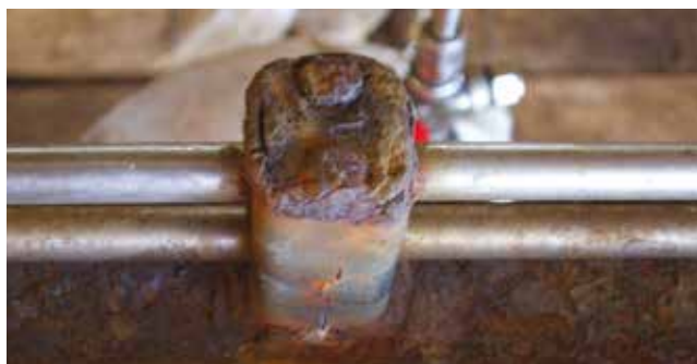
Crevice corrosion between the tube/tube trap interface.
