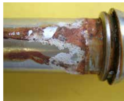
Picture of a low cost product. Corrosion damage created by a low quality hardening process applied to the back ferrule
